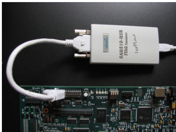
Figure 2-1. Connecting SAU510-USB ISO PLUS to target system and PC
